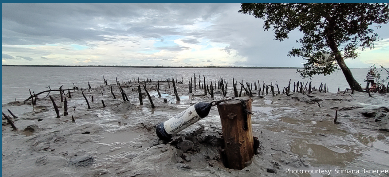
Mini Buoy in the mudflat of Indian Sundarban to characterise the hydrodynamics
